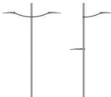
arms L=900 (double installation) single arm L=900 with intermediate
