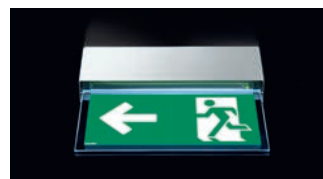
Indicator luminaire with Neutral White LED lamp, visible from a distance of 25 meters (EN1838), life 70,000 hours.
