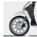
Static load resistance 1000 Kg
