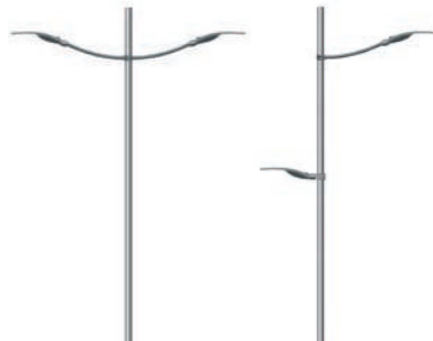
arms L=900 (double installation) single arm L=900 with intermediate
